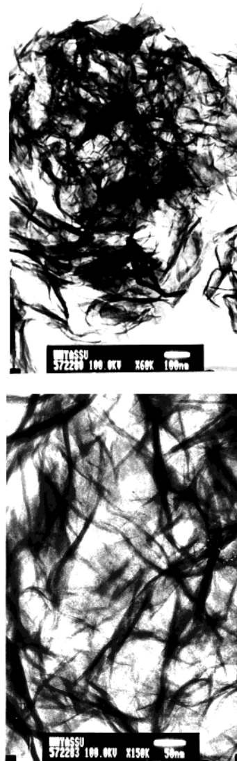
Figure 2. TEM picture of the sonochemically synthesized \alpha -nickel hydroxide at two different magnifications.
